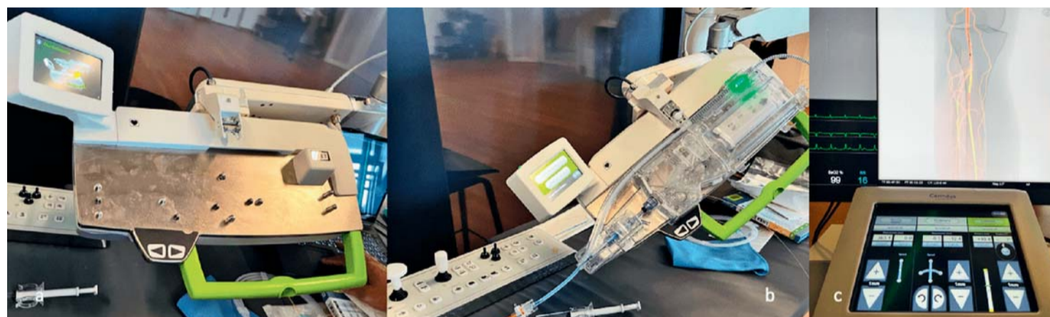
Figure 1: The CorPath GXR from Corindus Inc consists of a) a metallic arm that is fixed on the angiographic table, b) A "cassette" where the wires and the catheters are inserted, and c) a remote-control area of wire and catheter manipulation.
